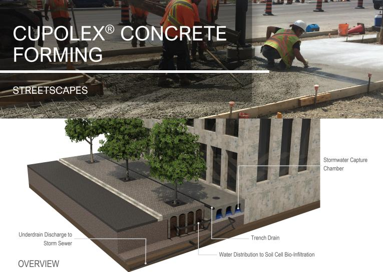
CUPOLEX® provides streetscapes with additional stormwater management properties. The concrete pavement designed by CUPOLEX® has voids underneath that are used to store stormwater and planting media. Due to its unique dome shape, the concrete is supported by a compacted base and does not rest on the planting medium. Stormwater is treated naturally through the soil. From there, stormwater can infiltrate to maintain a zero discharge site or be connected to a city sewer at a controlled rate.
