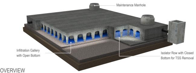
CUPOLEX® cast-in-place concrete infiltration structures eliminate the issue created with discharging stormwater off site. CUPOLEX® infiltration structures are designed with open bottoms in order to infiltrate the captured stormwater into the soil for natural treatment and to replenish local aquifers. It is a growing trend called Low-Impact-Development (LID) that involves managing stormwater at the source.
