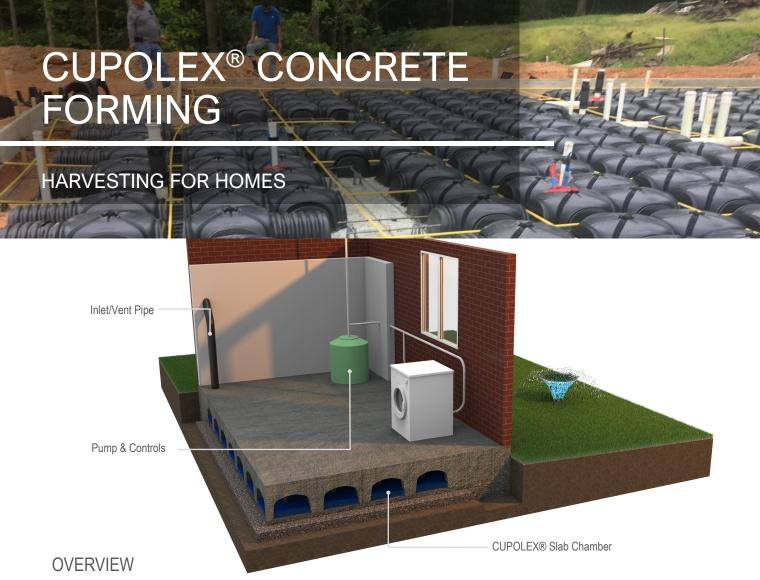
Residential houses and buildings can save potable water by harvesting rainwater, grey water, condensate and other on-site sources for non-potable uses like toilet flushing, irrigation and laundry. CUPOLEX® design engineering can integrate water harvesting tanks in any building structure or any single residential home foundation.
