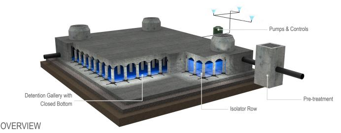
CUPOLEX® cast-in-place concrete harvesting structures and pavements provide cost-effective solutions for site applications where rainwater and/or stormwater needs to be retained for use on site. They also can provide additional detention capabilities for major storm events for slow release off site.
