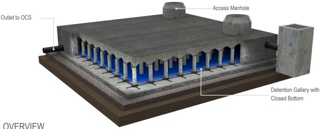
CUPOLEX® cast-in-place concrete detention structures provide cost-effective solutions for site applications where stormwater needs to be detained and allowed to discharge at a controlled rate.
