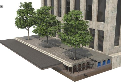
Can be designed with integrated stormwater capture, retention, infiltration, and treatment process as a stand-alone system.
