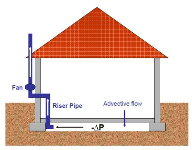
Figure 1. Conceptual diagram of an SSD system.
