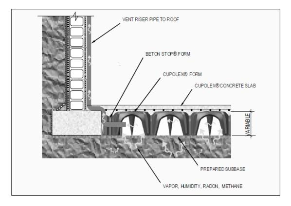
Figure 12. Typical riser pipe penetration with pre-existing footing
