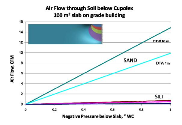
Figure 7. Modeled air flow rate versus negative pressure below floor slab.
