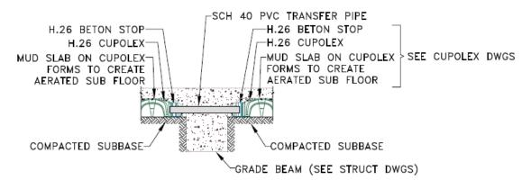
Figure 13. Typical detail for an air flow transfer pipe
