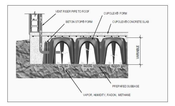
Figure 11. Typical riser pipe penetration into Cupolex void (suction point)
