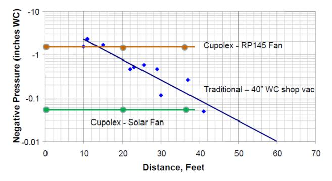
Figure 5. Negative pressure field data for a traditional and two Cupolex SSD systems.
