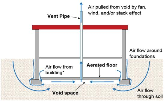
\*Through imperfections in seals, unsealed cracks, very minor for properly installed and sealed floors.
