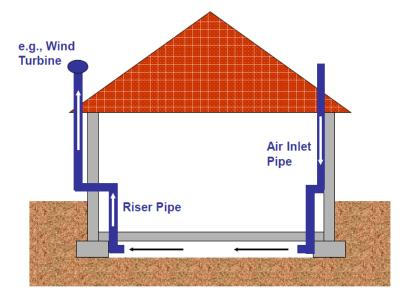
Figure 2. Conceptual diagram of a passive SSV system.
