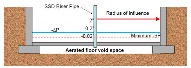
Figure 4. Negative pressure field with Cupolex floor SSD system.
