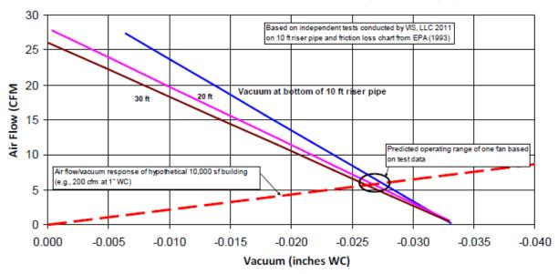
Flow vs Vacuum, Aura Solar Fan 4" PVC, (wind < 4 mph)
